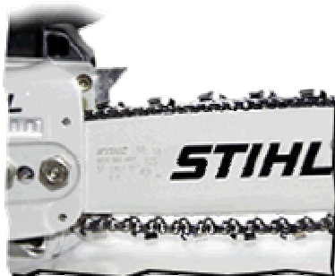
3. This chain is still too loose
